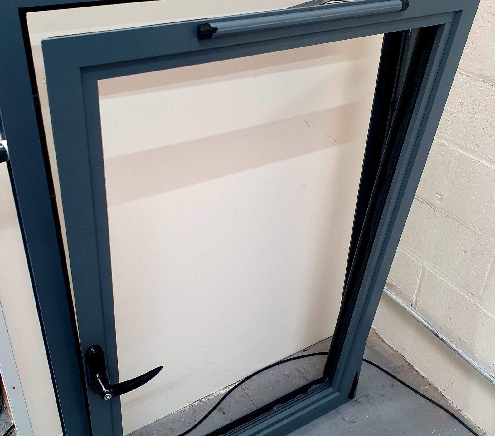
WORKSHOP SAMPLE Workshop verification of the actual tilt mode. The sash is unglazed here so the hinge geometry and top opening stay visible.
