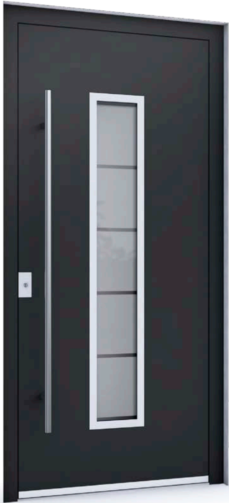
AP01 • AP 40.1600 door pull handle made of high-grade steel • Flush Alunox inlay; on the outside face • Glass pane: outer: VSG 33.1 middle: sandblasted with transparent strips inner: insulating glass with low-E coating • AP 3021 kickplate • AP 3400 anti-scratch protection • Surface finish: RAL 9005
