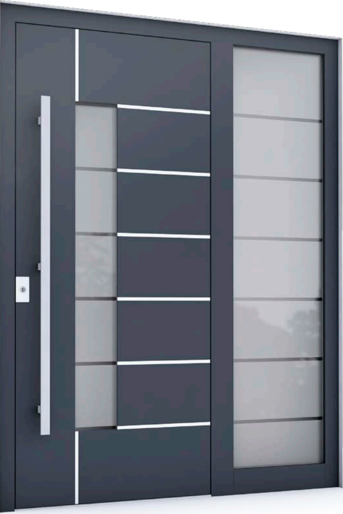
AP02 with a sidelite • AP 60.1600 door pull handle made of high-grade steel • Flush Alunox inlay; on the outside face • Glass pane: outer: VSG 33.1 middle: sandblasted with transparent strips inner: insulating glass with low-E coating • AP 3400 anti-scratch protection • Surface finish: RAL 7016
