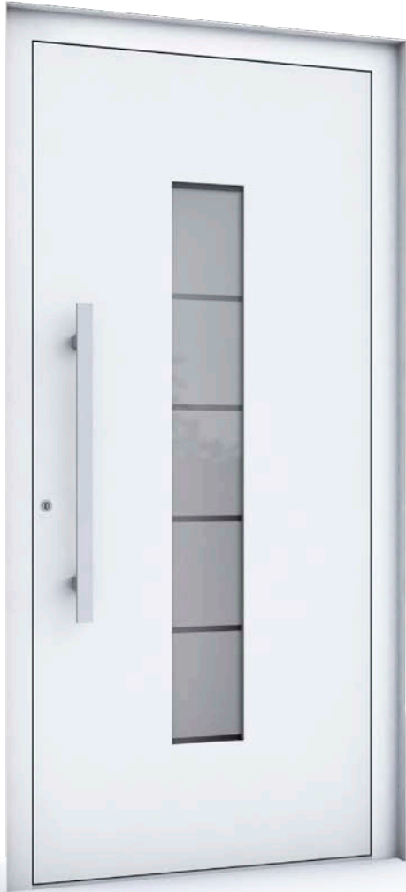
AP19 • AP 60.800 door pull handle made of high-grade steel • Glass pane: outer: VSG 33.1 middle: sandblasted with transparent strips inner: insulating glass with low-E coating • Surface finish: RAL 9016
